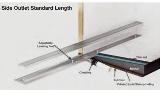
**STEP 3.** Pour a mortar bed across shower area, pitch at a 1/4" per foot slope in direction towards the shower base. Pitch begins level to the edge of the stainless-steel channel.
