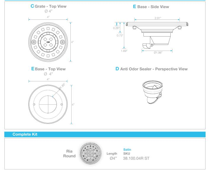
**Note:** Installer must verify all rough-in dimensions prior to installation and consult local and national codes. Conformity and compliance to local and national codes are the responsibility of the installer. Dimensions are subject to Manufacturers tolerance and change without notice. We can assume no responsibility for use of superseded or voided data.
