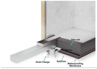
Before beginning installation make sure the distance between the center of the shower and the outlet is within 8" of each other
