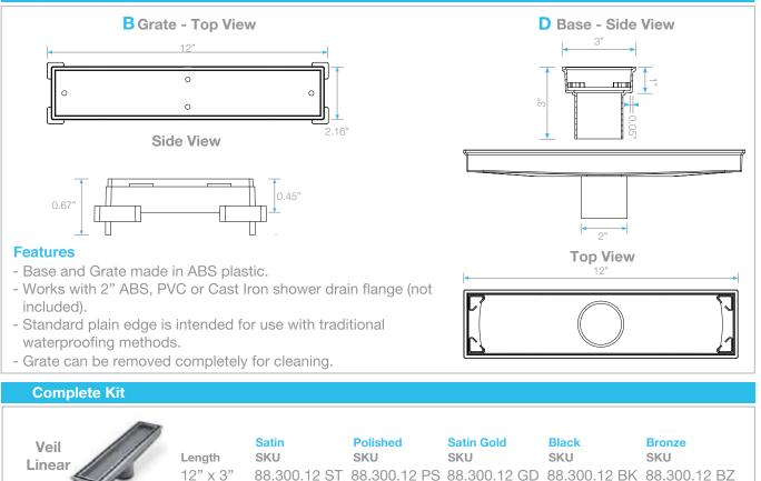
**Note:** If modern waterproofing method is intended using a bonded flange, add a bonded flange adaptor. See page XX Installer must verify all rough-in dimensions prior to installation and consult local and national codes. Conformity and compliance to local and national codes are the responsibility of the installer. Dimensions are subject to Manufacturers tolerance and change without notice. We can assume no responsibility for use of superseded or voided data.
