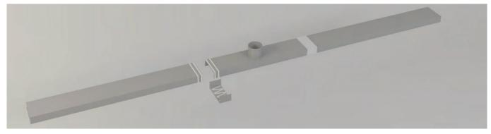
**Step 9.** Apply Sikaflex 1A sealant to trim pieces and fit them onto the longer outer edge of the channel. Remove any Sikaflex spill over. Allow to dry minimum of 8 hours before handling.
